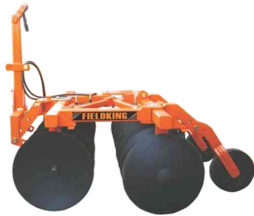
Dual Benefits Draw bar, Easy Mechanism for different soil condition, Heat treated boron steel disc, Inbuilt bearing hub for long life, Gang angle adjustable hydraulic cylinder (Optional), Gang axle lock
