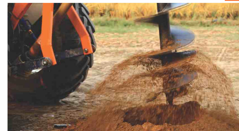
Semi double flighting auger
