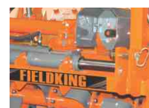
Hydraulic cylinder for side shifting with high strength chrome plated sliding arm
