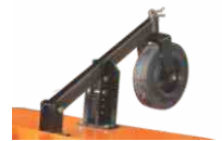
Tyre assembly for depth control
