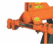
Hexagonal heavy duty drawbar
