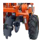
Side Drive Wheel for Power Transmission
