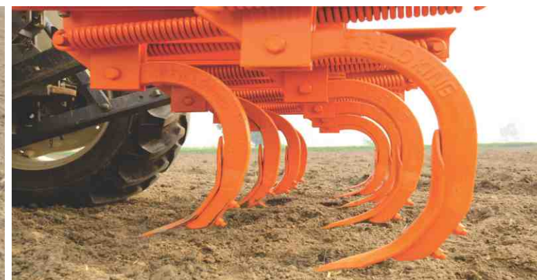
Spring having more capacity of absorbing shock
