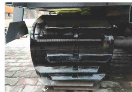
Wider track 500 mm x 90 mm (WxH) Number of grooves 56
