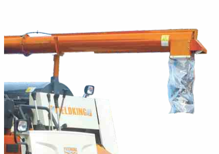
Quick discharge at 340° rotation at variable height
