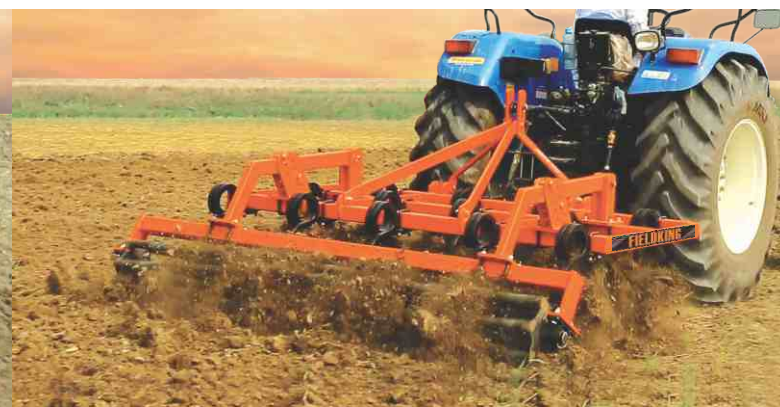
Double coil spring action tyne
