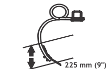
225 mm (9") Double coil tyne of EN-45 material
