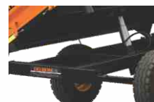
Tubular structure Chassis
