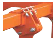
Tyne mounting clamp & shear bolt
