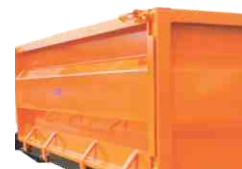
Corrugated sheet for strength
