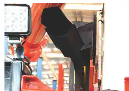
Vertical exhaust system
