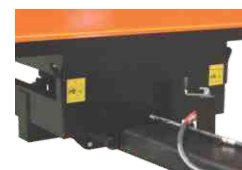
Detachable drawbar for increased loadability
