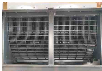
Axial flow technology of thresher which is of size 1.95m.
