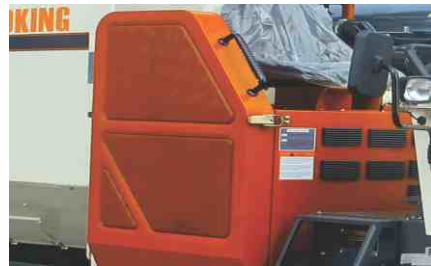
Protective dust cover for efficient radiator cooling
