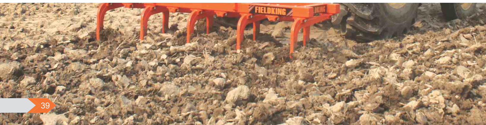
Unique tyne design to absorb shocks at stress prone area
