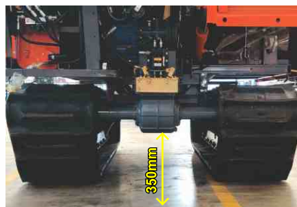
Higher ground clearance (350mm)
