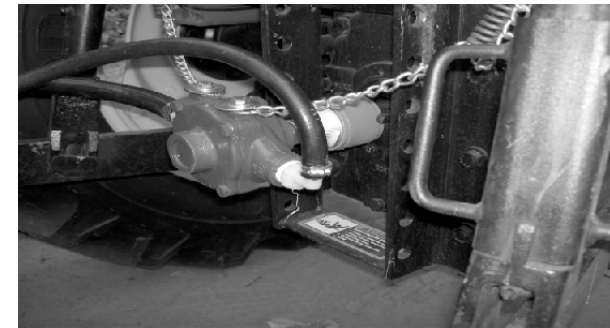
Photo of the sprayers pump connected to the tractors PTO.
