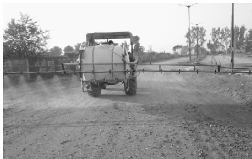
Photo showing the boom fully unfolded in spraying position.
