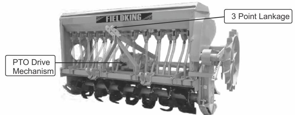
Hitching of machine through three-point linkage.
