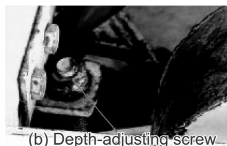
Fig 15. Depth-control side wheel (a) and depth-adjusting screw (b).
